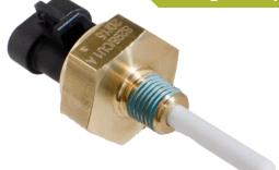
The **S298** is an active device designed to give an alarm signal if liquid falls below, or rises above, a preset level. It can be specified with a delay to eliminate false alarms due to turbulence.
