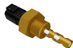
The S284 is an active device designed to give an alarm signal if liquid falls below, or rises above, a preset level. It can be specified with a delay to eliminate false alarms due to turbulence.
