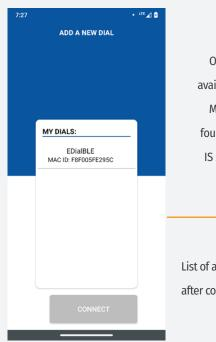
Once the App has completed scanning for available e-Dials<sup>™</sup>, they will be displayed by MAC ID. The MAC ID of the e-Dial<sup>™</sup> can be found etched on the dial bezel or top of the IS safety barrier box. Select the e-Dial<sup>™</sup> to connect to and select "Connect"
