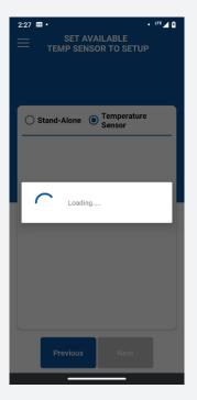
2. Once Temperature Sensor Option is Selected, App will promptly scan for nearby available Temperature Sensors to connect to. Please allow the app to complete scanning before selecting Temperature Sensor to connect to
