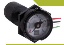
The **G/LL65** vertical spiral gauge is a mechanically operated liquid level gauge with a local display and two electrical outputs. Suitable for connection to a typical controller or remote level indicator the outputs are; a variable resistance proportionate to the liquid level and a volt-free switch to trigger an alarm when the liquid reaches a prescribed level.
