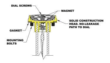
The Rochester magnetic liquid level gauge operates simply by means of a float actuating a powerful magnet inside the container which in turn provides an invisible "magnetic coupling", through a solid head, with the magnet on the pointer in the dial chamber. Thus the gauge head completely seals off the liquid in the container so the dial may be removed and replaced quickly anytime without loss of liquid.
